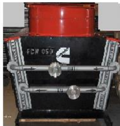
Remote radiator for Secondary circuit
